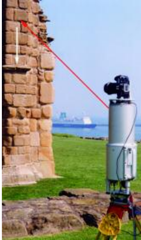
Fig 16 A time-of-flight laser scanner, showing measurement beam and direction of scan (courtesy of Riegl UK).
