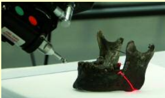
Scanning of the lower jaw fragment with ModelMaker X laser scanning.
