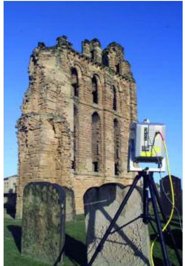
Fig 2 (left) Triangulation laser scanning (courtesy of Conservation Technologies, National Museums Liverpool).
