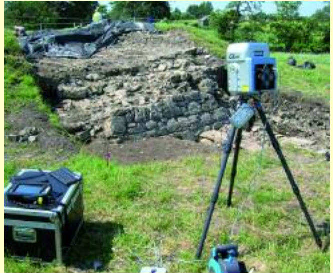
The Mensi GS scanner set up among the masonry remains of the tower.
