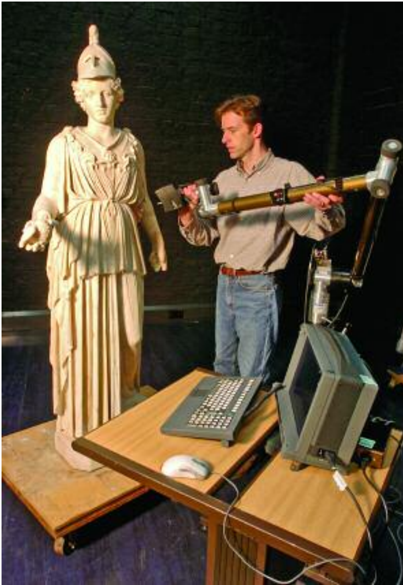
Fig 2 (left) Triangulation laser scanning (courtesy of Conservation Technologies, National Museums Liverpool).
