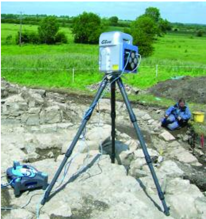
Fig 9 Using laser scanning to contribute to a record during excavation (courtesy of the Discovery Programme Ltd).
