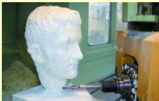
The replica during CNC machining.
