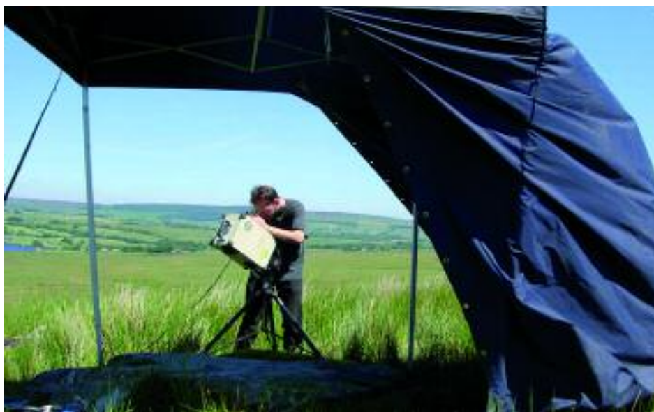
Fig 13 (above) Triangulation laser scanning of rock art, on site with a canopy to reduce the influence of bright sunlight (courtesy of Tertia Barnett).
